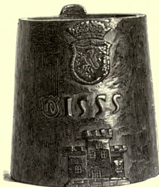
FIG. 235. Standard choppin or half-pint in the custody of the City of Edinburgh.
